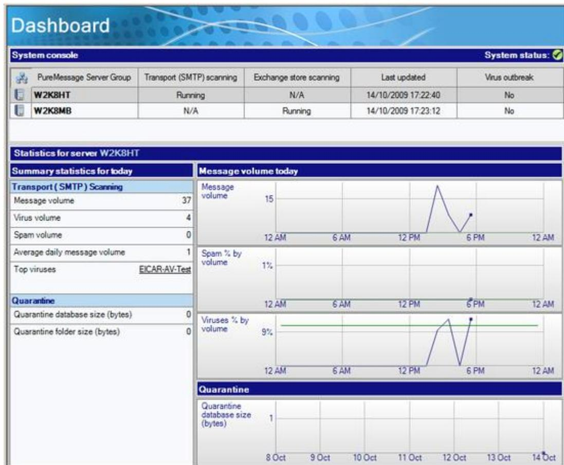
By default, the servers are listed in alphabetical order on the dashboard, unless one or more registers a system failure. In this case, the System Status traffic light becomes red, the faulty server is marked with a warning icon, and the server is displayed at the top of the list.
