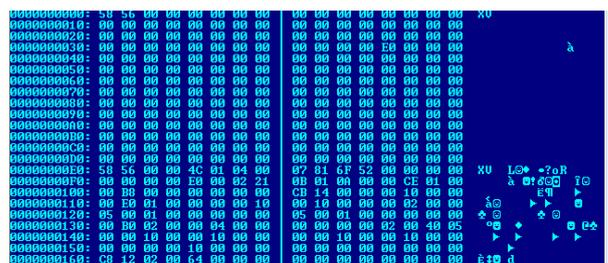
Fig. 3. Note the beginning of the file is missing the PE designation, in an attempt to evade detection.
