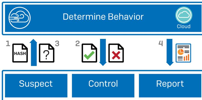
1. The Sophos security solution scans files against all conventional security checks (e.g., anti-malware signatures, bad URLs, etc.). If the file is executable or has executable content and is not downloaded from a safe website, the file is treated as suspicious. The Sophos security solution sends the suspicious file hash to Sophos Sandstorm to determine if it has been previously analyzed.
