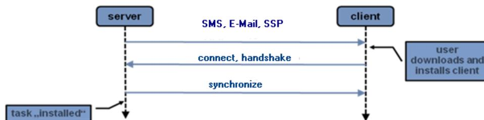
After client installation specific information of the device is collected and sent to the server during the first synchronization process.
